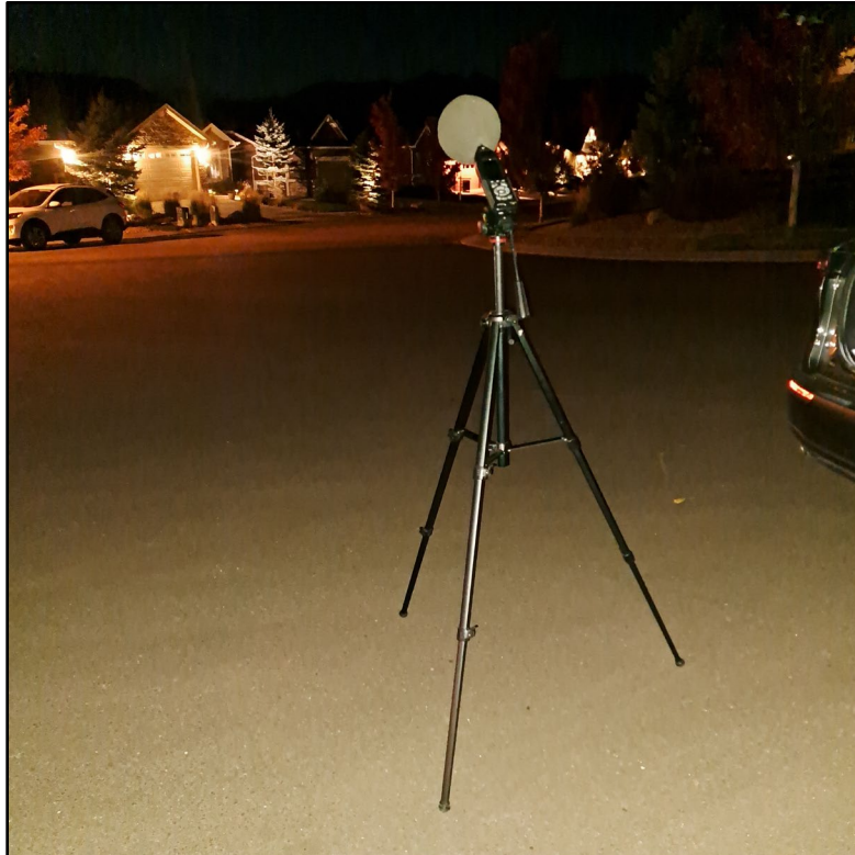
Figure 1-3. Typical Community Sound Level Measurement Setup
